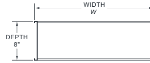
MODEL: ACL800 FRAME: CHANNEL FRAME DUCT-MOUNT (DM)
